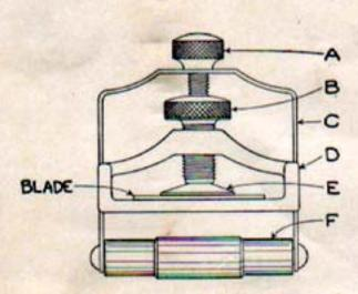
By turning the knurled angle adjusting screw "A," adjust position of the Blade Bed "D" so that its bottom is about 3/8" from the Roller Bearing "F."
