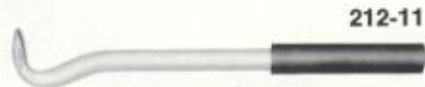
Nail Puller. Hot forged, heat treated tool steel with 3/16" hex shank. Non slip cushion grip handle.
