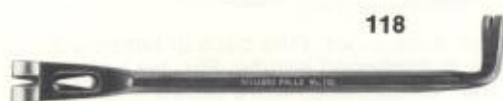
Offset Chisel. 90° offset chisel claw for pounding, angle chisel prying claw with three beveled nail slots for powerful prying. Drop forged tool steel, with heat treated shank ends.
